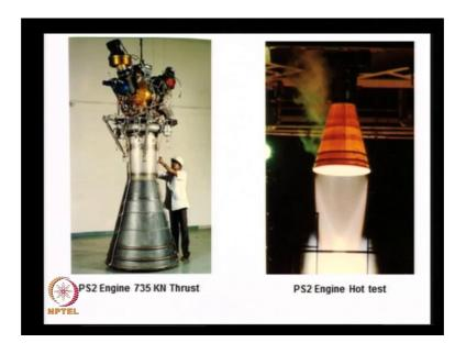
Let us take a look at few liquid propellant rockets. Well, this is the thrust chamber of the liquid propellant rocket engine, which was seen earlier. It is taller than this man over here, this is the cylindrical combustion chamber, this is the pump above it, this is the nozzle and this slide shows the rocket firing.
