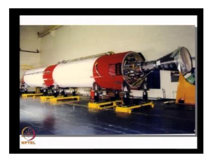
Well, the same engine assembled together as a rocket stage is shown with large tanks to carry fuel and oxidizer. We have the oxidizer tank over here, I have the fuel tank, I have
