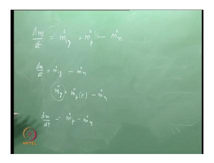
We would like to solve the mass balance equation. We say the rate at which mass is added by the igniter; during the process of flame spread, mass is not only added by the igniter and also the ignited burning surface area is also adding mass as the flame spreads. We are adding more and more mass as the more of surface of the propellant is getting ignited.
