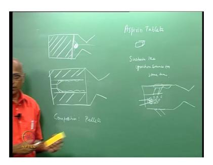
We have a solid propellant in an end burning configuration; we have the nozzle over here downstream of the grain. We want to ignite it. From the nozzle side we introduce a bag of pyrotechnic charge, inside the bag we have a squib; we ignite the pyrotechnic charge over here, a flame is formed and it impinges over the surface of the propellant and the surface catch fire.
