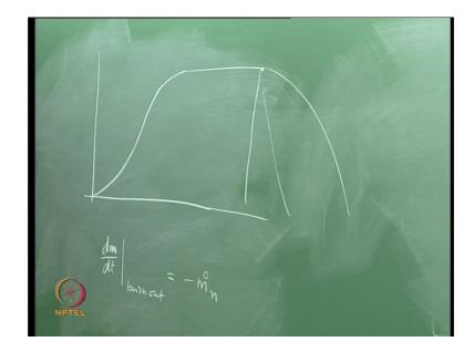
When we ignite a solid propellant rocket, we know how to calculate the equilibrium pressure and the transient during ignition. When the rocket ceases to burn, how does the pressure fall? And we use the same theory again.
