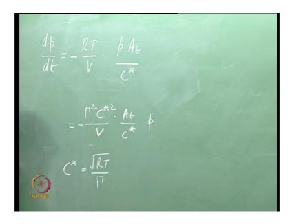
Let's let us solve this equation. We have  $dp/dt = -RT/V \times p \times At /C^*$ . The product of RT can be written in terms of C\* since C\* =  $\sqrt{RT/\Gamma}$ . Therefore, we substitute  $\Gamma^2C^{*2}$  for RT. This is divided by V and multiplied by At and divided by C\* and multiplied by p.
