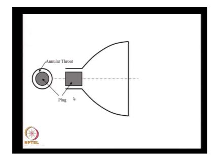
Those who are interested should go through it. This is a plug nozzle. I put a plug in the throat to make an annular throat. We have an outer surface, which guides the flow. The inner surface is free therefore, it can adapt to the ambient pressure. What you have is an annular throat, instead of having a cylindrical throat.
