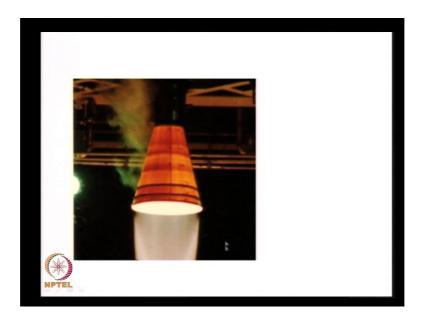
I repeat the case of a hot nozzle in this slide. A nozzle is firing for a certain amount of time. This is the conical nozzle. You see, that the nozzle runs red hot.
