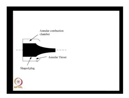
This is what we called as a plug nozzle or a spike nozzle. We have a spike following the annular throat. The flow comes from the annular combustion chamber. The hot gas is generated in an annular chamber instead of a cylindrical chamber. We push the flow onto this inner contour surface and this surface guides the flow. Outer surface is free; therefore, the expansion can adapt to the altitude. It is not used in practice. This summarizes what we learnt about nozzles.
