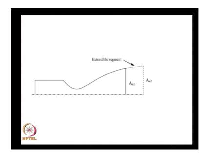
Initially, we have a small area ratio corresponding to exit area  $Ae_1$ .We store another segment on top of this a segment between area ratio  $Ae_2$  and  $Ae_1$  and at higher altitude deploy or push itto get the larger area ratio nozzle.
