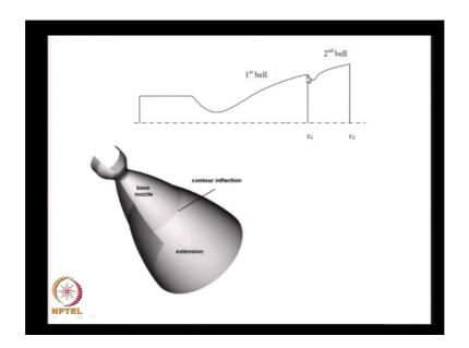
This is a dual bell nozzle. As you see along the divergent contour we have a step at which for higher ambient pressure the flow separates but at lower ambient pressures follows the contour of the second part of the nozzle. As I told you, there was a research paper in the AIAA Journal this month in which dealt with the dual bell nozzle.
