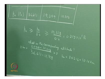
This works out to be something like 8 plus 2.16 which is equal to 10.16 kilometres. Therefore, this is the altitude at which flow separation ceases or thereafter the nozzle is either runs full or is under expanded. This is all about nozzles.
