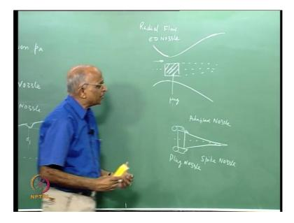
Therefore, what we have done is, we have introduced a plug in the throat region and we allow the contour to change the pressure of the outer flow. But, the inner region of the flow is keept free to expand. This is the principle of the expansion deflection nozzle.
