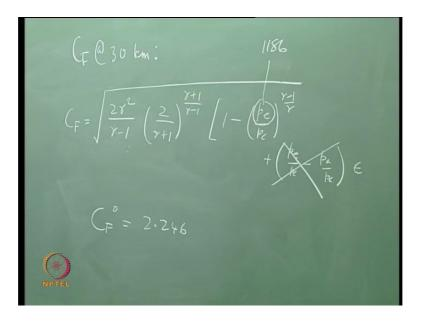
Well, pe must equal to pa. Therefore, for optimum, this term will get knocked out and what will be the value of pe, if it is optimum. Take a look at this table. Optimum at 30 kilometres, that means, I will have a nozzle which gives me this value, 1186 Pa. Therefore, I now change the value of pe as equal to 1186 and the pressure term is no
