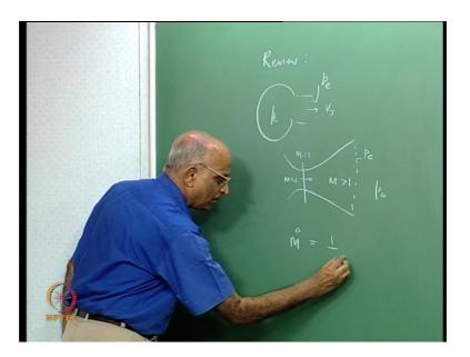
We called this nozzle as a de Laval nozzle or a convergent divergent nozzle. In the convergent part, the Mach number was less than 1; in the divergent the Mach number was greater than 1. After having done this, we said at the exit I have exit pressure which
