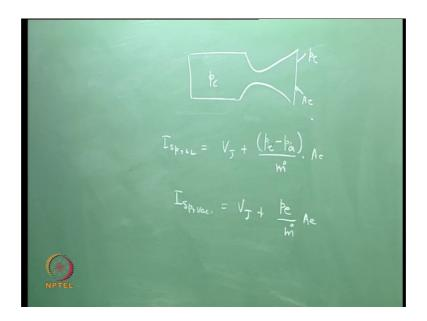
Now, what would be the value of specific impulse for the same nozzle functions in vacuum; I call it as vacuum specific impulse. Vacuum is equal to what would be the value of pa; it is 0. Therefore, we have  $V_J + (pe/m^\circ) \times Ae$ . In other words, the same nozzle when it is fired in vacuum gives me a higher thrust because, minus pa is missing in the above expression. Can we relate these two?
