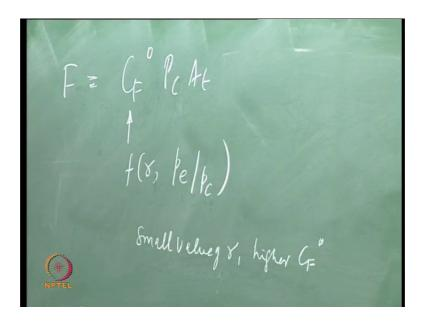
Therefore, we have looked at the thrust coefficient for optimum thrust viz., when you have a case of Pe = Pa, for which the thrust  $F = C_F^0 \times Pc \times At$ , we find that the value of
