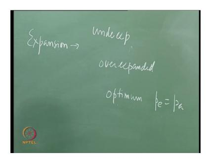
And when we get a diamond pattern it is of interest to see that whether it is due to underexpansion or over-expansion in the nozzle. The optimum is when the exit pressure of the nozzle is equal to ambient pressure in which case it goes straight without the formation of the shock diamonds.
