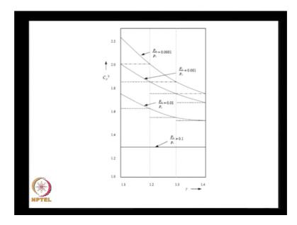
The same results are plotted on this particular slide, wherein the optimum thrust coefficient is shown as a function of  $\gamma$ . We find that at large values of Pe by Pc,  $\gamma$  does not influence the thrust coefficient  $C_{F0}$  coefficient at all. If we have a small values Pe/Pc, variations in  $\gamma$  cause a considerable change in the thrust coefficient. That means, a decreased value of gamma will give us a higher value of  $C_F^0$ .
