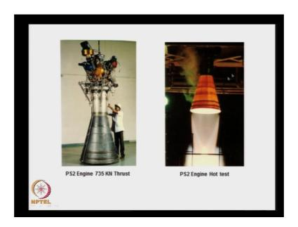
See in this case, we have oblique shock wave at the nozzle exit and the plume is seen to collapse inward. The shock diamond is formed a little later as is seen here. But in this particular test water is used for cooling the plume so that subsequent shock diamonds were not visible.
