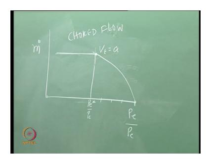
In this experiment, we plot the mass flow rate through the nozzle, that means, the rate at which mass is getting sucked out as a function of let us say the value of Pe that is the exit pressure to the chamber pressure as it is progressively decreased by the running of the vacuum pump.
