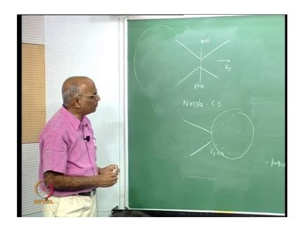
If we want to have a high value of jet velocity, it is essential for us to have a convergent followed by a throat section, followed by a divergent section, with the condition that the Mach number must be one viz., velocity must be equal to a sound speed at the throat. And with this condition the velocity keeps increasing. We can get a high jet velocity at the exit and this is what the convergent divergent nozzle does.
