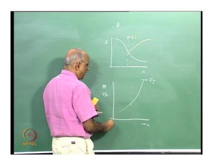
Therefore how would the sound speed vary occur along the length of the nozzle? Well the sound speed starts with a high value of sound speed corresponding to the high chamber temperature; it keeps on coming down and it like this along the length of the nozzle as the temperature drops.
