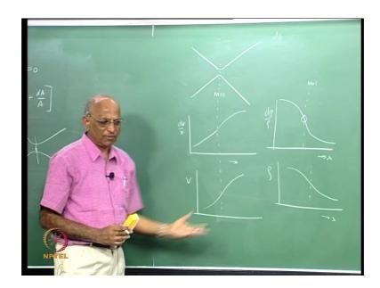
Let me first sketch a nozzle, converging till the throat, followed by a divergent and let us assume that the flow rate through the nozzle is such that the Mach number is equal to one at the throat. Now, let us first find out what is a change in dV by V along the length. We just now saw that dV by V increases up to the throat since the Mach number is less than one and the variation in dA is negative as x increases.
