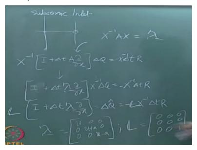
So if I look at the left boundary and I look at a subsonic inlet, so these are the subsonic inlets and subsonic exists are the interesting one, inlet, I look at the subsonic inlet, so this is the interface at the inlet. So at this point, at this grid point I have one I have this equation I coming in from the left hand side + delta t, now what I am going to do is over this small interval that I have between these few grid points.
