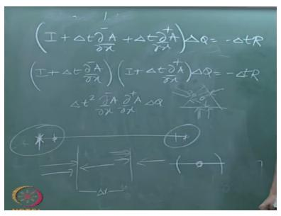
So the—if you remember LU approximation factorization we wrote it as dou/dou x-2 operators, split it as 2 operators acting on delta Q is -delta t\*R. And this can be factored, this can be factored as, this can be factored approximately as I+delta t A dou/dou x acting on delta Q=-delta t\*R. Okay. So this derivative would involve the grid points P and P-1; this derivative would involve the grid points P+1 and P. Okay.
