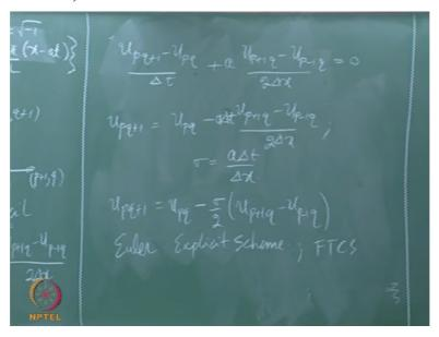
So, do we have substituting into our governing equation. So you have Upq + 1-Upq/delta t + a times Up + 1q - Up-1q/2 delta x, should be approximately 0 we set it = 0. And this is the objective, this is what I am trying to get. This is the objective. The objective is Upq + 1 then we written as I take everything else note this is only one that is the time level q + 1. All of these are our time level q.
