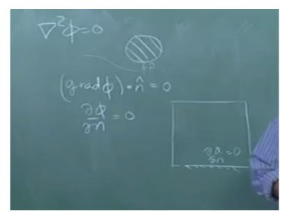
So normally when we do flow past anything, flow past cylinder or something of that sort, right, I just set up the boundary conditions and then we will talk about it later, so and we have Laplace equation for so if you say the flow is rotational, so I would not go through the fluid mechanics of all of this, right, so if this is the solid cylinder and there is a fluid flow past the cylinder, there is a flow past the cylinder, okay.
