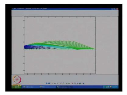
This I have to explain it to you little bit, you are seeing that the set of compression waves coming from there from the pressure boundary, you can see that I am showing only the nozzle exit from here, and then expansion wave is shown in saint color light blue. And then the green is characteristic coming from the pressure boundary point, you are seeing that the pressure boundary or the jet boundary itself is turning downward.
