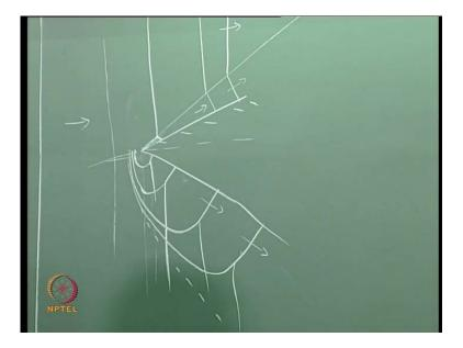
If I have a wedge flow, and I am saying that I am having a supersonic tunnel just now beginning to have a flow, that is the starting normal shock just now traveling through. How will the flow field develop around this body, till now there was no flow or very low subsonic flow, suddenly there is supersonic flow coming and it is always leading there will be a leading shock that is your starting shock of your tunnel.
