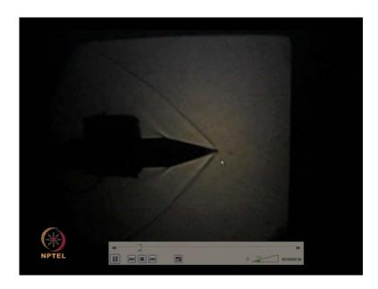
This is flow the other way, here you could have seen the shock moving slowly, here you can also see the expansion fan, and also the mach waves you are seeing thin lines coming in from this sides. The way we got the thin lines here and here, etcetera are by putting thin grooves on the nozzle, so we use that to form these thin lines will look at more next class see you people.
