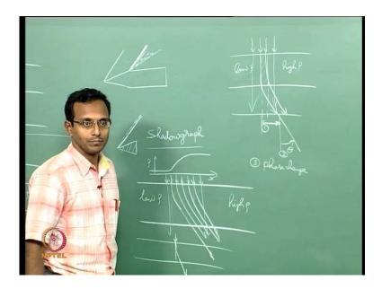
Now I am seeing new things I am seeing some other region I will draw this picture again here, initially I will just be seeing this shadow, but because of shock being along this line I will draw thin line. If this is the shock I am going to have, I will draw a dotted line and the solid line, I am going to get a line where it is dark and the line, where it is bright.
