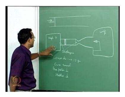
Then I go back to this picture and I will say here, I will put combustible measure. T hat will create higher pressure and temperature that will rapture the diaphragm 1 and then it is going to operate like a free piston tunnel. That is also a possibility when it will become combustion driven free piston tunnel.
