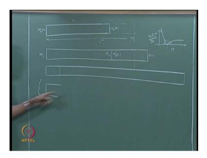
With this idea exist wanted to re iterate this whole thing in one sequence, want up I will start with M l equal to 1 in here, M l equal to 1 I cannot send M l equal to 1 flow into any duct because, immediately after that there is be a friction which will send compression waves, which will slow down the flow and immediately we will get only a subsonic case behind, that is why transonic problem is very, very difficult it could
