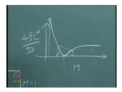
This particular curve is starting to turn around 0.3 plus it will start turn steeply, initially it was out there now, I slowly turning, turning, turning that turning point start seriously only after 0.3 mark number, above 0.3 mark number there is more sensitivity to mark number. And when we are going very close to M 1 there is lot more change to it.
