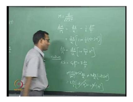
Let us find out that next what do we have M equal to u by square root of gamma RT. So, now, I can tell that I will just go a little faster dM by M equal to d u by u minus 1 by 2 dT by TI am assuming you can do that one more intermediate step just differentiate this and divide by M you can do that you will get to this particular form.
