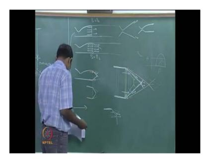
This is my nozzle exit edge, 1 edge only. I am showing there is a shock and that is reflecting like this with a normal shock. Here if this is happening there locally the fluid boundary is this. I will erase the extra things and below this line, fluid is just seeing a normal shock. It just jumps like a normal shock. The remaining region is going to come straight turn like this and go like this.
