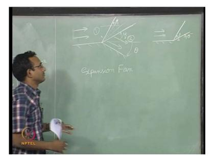
We will come back to the one d expression later if there is a supersonic flow going like this previously when we did shocks we remembered this basic flow shape last class I told you right this is your reflection of the wall is into the field flow is coming like this the wall moves into the flow the flowand this becomes the compression wave whole bunch of compression waves come together to form and contrast.
