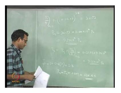
I want to find P naught by P for M equal to 3, how will I do it, if I do it by formula it is going to be 1 plus 0.2 into 9 to the power, gamma by gamma minus 1 is 3.54, gamma equal to 1.4. I just have to find this number, it is what, 1.8 2.8 to the power 3.5, that number happens to be 36.73. If I go look at the tables also, I will get the same number, isentropic tables for M equal to 3 will give you this number, if you go to gamma equal to 1.4 tables.
