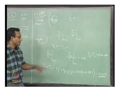
I am having a cylinder, we are looking at a 2D problem, this dimension is infinite, minus infinity to plus infinity. And this is moving at Mach 2 what does that mean, if I shift my reference frame to this on the cylinder then I will remove this arrow here and I will say, my flow is coming in with free stream Mach number of 2 this is what, we are having. And as I already told you, if I put any object in flow in supersonic flow, there will be a shock in front of it.
