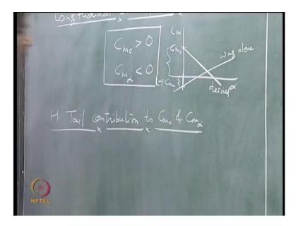
So, in this class, we will continue with our discussions on longitudinal static stick fixed stability of the aircraft. We will discuss an airplane to have stability in pitch and also to be able to fly at positive angles of attack, it should satisfy two condition or rather it should have two properties and they are  $C_{m0}$  which has to be positive and  $C_{m\alpha}$  must be negative.
