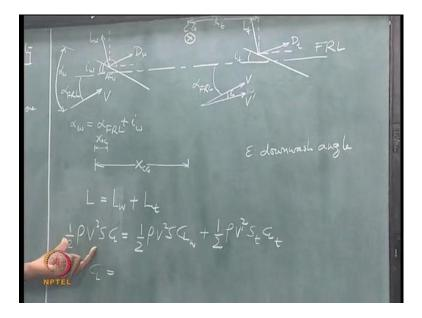
So, let us say this is our fuselage reference line (Refer Slide Time: 5:51). The wing is located here and relative wind is coming onto the aircraft at an angle of attack which is measured with respect to the fuselage reference line, and therefore, is called  $\alpha_{FRL}$ . So,
