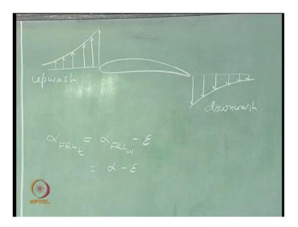
So, the flow field around the wing will look something like this. This is downwash, this is upwash. How is angle of attack going to change at the tail now because of this downwash? So, alpha FRL  $\alpha_{FRL}$  at the tail is going to be  $\alpha_{FRL}$  at the wing minus this
