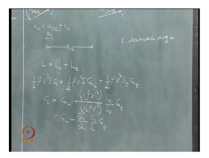
You can divide the right side by this quantity (half rho V squared S  $\frac{1}{2}\rho V^2 S$ ) you get, so, you can also write this as Sw  $S_w$  because wing planform area is the one which I am using as reference area. What is this quantity (Q t over Q w  $Q_t/Q_w$ )? This is the ratio of two dynamic pressures.
