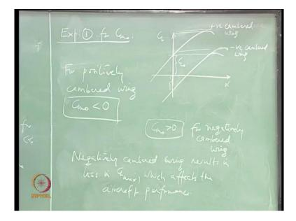
Now, expression 1 for  $C_{m0}$ , let us look at that. So, this quantity ( $C_{m\alpha}$ ) has to be negative because we have to ensure stability. So this is negative and what we want is  $C_{m0}$  must be positive. So,  $C_{m0}$  positive is the condition to fly the aircraft at positive angle of attack and which we would want for several reasons, because negative angle of attack is going to result in negative lift (for symmetric airfoil).
