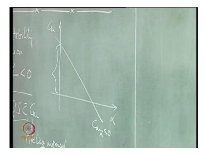
We will continue today from where we left on static stability. We were talking about longitudinal stick fixed static stability. The criteria for this is related to stability in pitch, we can also call it pitch stability. So, if you remember, we said an aircraft to be statically stable in pitch has to have Cm versus alpha curve which has a negative slope. This was the criteria for pitch stability.
