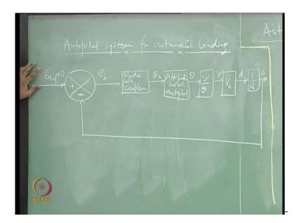
The reference variable here is the deviation angle which has to be 0. Error in delta ( $\delta$ ), the deviation angle is fed to what is called glide path coupler which is trying to change the attitude of the aircraft, so that it is following the glide path. And here, an altitude hold autopilot is engaged because (so that) theta can be maintained at the prescribed value. This will change the flight path angle according to this dynamics. This gives gamma ( $\gamma$ ).
