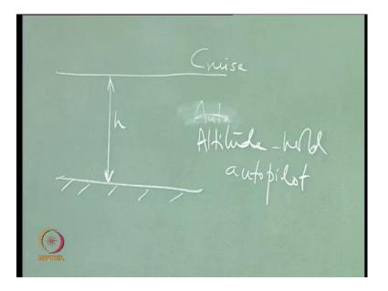
Autopilot systems are mainly used to keep the aircraft on a prescribed path or attitude. What you want to do here is, design a control system such that, for example, you know this height (Refer to the sketch) is maintained throughout constant in flight; as in cruise.
