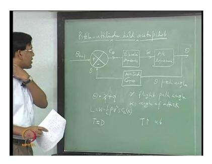
The idea actually can be represented using this schematic, which is also called block diagram. So, this is about controlling the pitch angle, theta ( $\theta$ ) is the pitch angle here (Refer Slide Time: 10:30). This is the reference theta ( $\theta_{ref}$ ) at which we want to keep the aircraft at all times, even in the presence of disturbances.
