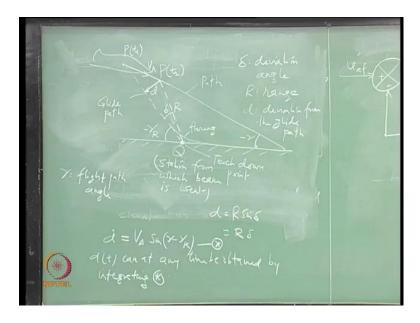
This equipment or the station from where the beam is thrown, is this. An aircraft which may be following let us say this glide path. Let us say, this aircraft is following this path; not really in a glide path and it is supposed to follow this beam. This (the dashed line) is actually the glide path and this station is at touchdown point, and after which the aircraft has to flare out and then move on the runway for some distance before it stops. This (curved path) is called flaring.
