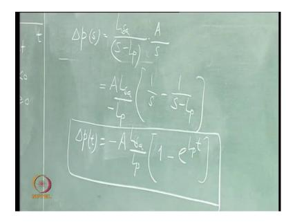
So now if I do that I can find out what delta p is in terms of time. Delta p t equal to minus A into L delta over L p into 1 minus e raised to L p into t ((audio not available refer time: 37:43 to 38:13))  $\Delta p(t) = -A \frac{L_{\delta a}}{L_p} \left[ 1 - e^{L_p t} \right]$ . Clearly it depends upon this Lp, Lp also gives
