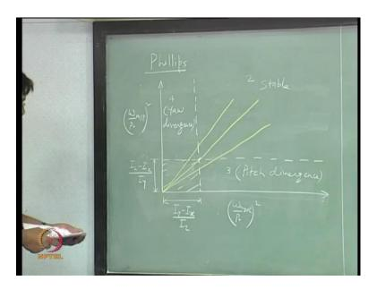
((No audio 18:48 to 19:12)) So, this boundary is defined in terms of this ratio, ratio of short period frequency over the steady roll rate squared  $(\omega_{nSP} / p_0)^2$  and Dutch roll frequency over steady roll rate squared of that,  $(\omega_{nDR} / p_0)^2$ , and using the conditions that we have, based on the inertia terms and these frequencies ((no audio)). .....
