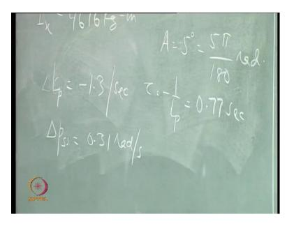
Trim speed is given .... ((no audio)) This is a solved example in Nelson. What other things are given are: this  $C_{lp} = -0.285$ . Cl delta a  $C_{l\delta a}$  is 0.039. *S* is 18 meter square and *b* is 6.7 meter and, *Ix* is 4676 kg-m square. So, *A* is 5 degrees; *A* is the amplitude of the step input in aileron. So, *A* is 5 degrees which is 5 into pi over 180 radians, and  $L_p$  you can find out using that formula, ... it turns out to be minus 1.3 per second.
