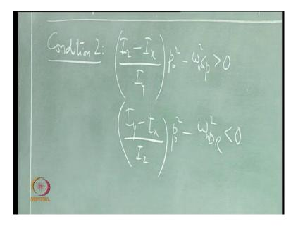
((Audio not available refer time: 16:36 to 17:22)) These are two conditions for instability and we look at the parameters that are involved. Parameters involved are inertia terms and the frequencies of short period mode and the Dutch roll mode. Rolling maneuver is considered to be a fast maneuver and the instabilities are also are due to mainly inertial coupling terms.
