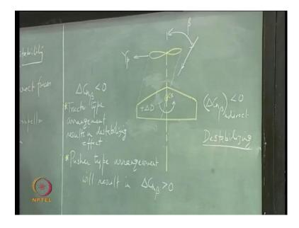
So, let us say the propeller is rotating, right, and there is an unbalanced force because of this propeller, which is in the negative Y direction right, and this force can be, because of this side slip angle. So, which way it is going to create a moment, negative yaw moment.
