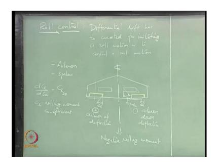
So, you know that to initiate a roll motion or control a roll motion, you have to create differential lift over the two sides of the wing.
