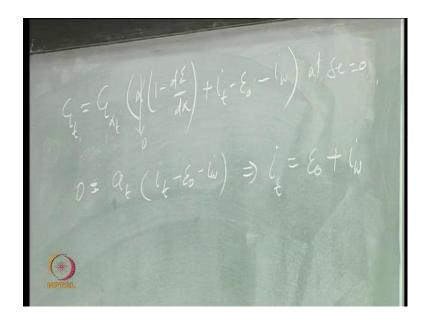
$$C_{Lt} = \underbrace{C_{L\alpha t}}_{a_t} \left( \underbrace{\alpha}_0 \left( 1 - \frac{d\varepsilon}{d\alpha} \right) + i_t - \varepsilon_0 - i_w \right) @ \delta e = 0$$
