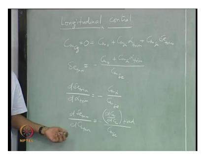
$$C_{mCG} = 0 = C_{m0} + C_{m\alpha}\alpha_{trim} + C_{m\delta e}\delta e_{trim} \Longrightarrow \delta e_{trim} = -\frac{C_{m0} + C_{m\alpha}\alpha_{trim}}{C_{m\delta e}}$$
