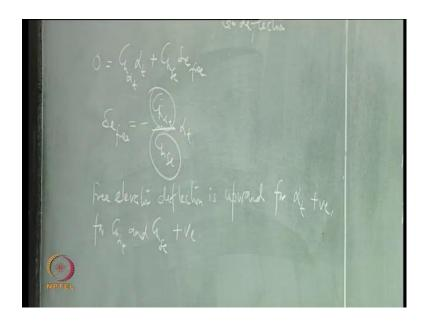
$$C_{h} = 0 = \underbrace{C_{h0}}_{0} + C_{h\alpha t} \alpha_{t} + C_{h\delta e} \delta e_{free} \implies \delta e_{free} = -\frac{C_{h\alpha t}}{C_{h\delta e}} \alpha_{t}$$
