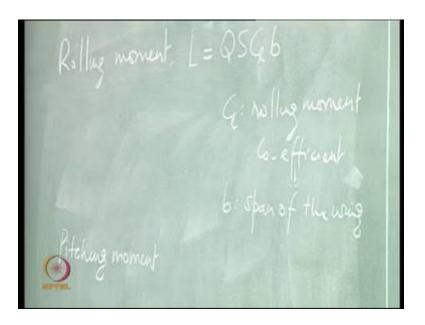
These moments are: rolling moment, the expression for which is, L is the rolling moment, the sum of all the (aerodynamic) moments acting about the X axis of the aircraft is rolling moment. So, everything else you know, Cl is the rolling moment coefficient and b is the span of the wing.
