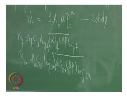
Because pc goes as 1/1- n so therefore if you look at solids this is how the masses mass is generated and if you look at liquids, liquids the m dot is given as a CD a injector this is mass of injector so mass of fuel so I will put this S and similarly you will have oxidizer also the N here indicates the number of injectors okay.
