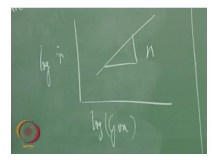
So the overall mass burn rate m dot shell in this case would be now a is nothing but justice and solid Rockets we had a there which we said is the burn rate at unit pressure this is also the burn rate at unit mass flux okay so what is typically done is we plot r dot vs 0 x on a log-log scale therefore if you on a log-log scale if you get a straight line then the slope of that straight line will give you n okay.
