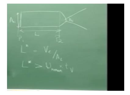
If you remember AP right AT we had got from what considerations thrust and mass flow-rate considerations right. This is fixed then what we are left with is how to design this length of the motor and what should be the cross-sectional area of the motor or the engine. In this case so this is AC and this is length if you remember we had defined something called L star with respect to solid rockets right.
