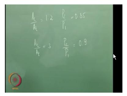
So if we have different AC /AT if we have AC/ AT= 1.2then P 2/ P 1 this ratio would be 0.85 and if we have AC / AT= 3 will be larger because you now have an larger area to have a mass flow
