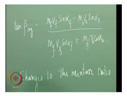
So if we calculate the tan of the angle  $\beta$  injector this can be expressed as this is from purely momentum balance now if due to any reason the mass flow-rate or one of the parameters of one of the Jets varies then the resultant direction will also change which is not a very good thing right it will also result.
