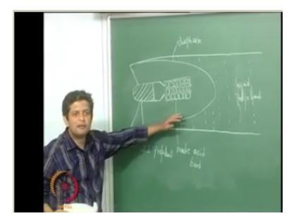
So let us say you have solid propellant only a converging nozzle is good enough here because you do not want too much of a pressure drop you are not interested in velocity here you are only interested in pressure and then if you have a chamber which has this oxalic acid pellets then the exhaust of this can be connected to the or let me do that also let us say you have this at the head end of the tank right.
