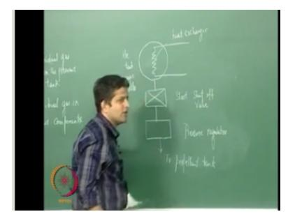
And one of the designs to overcome this is to have in the helium tank itself a heating this is a heat exchanger okay if you have a heat exchanger here ask the helium cools down if you supply heat to it then the temperature would not drop so much and therefore you will have a lot more of useful pressure okay there is one way of doing it.
