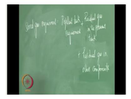
So the stored gas requirement is equal to propellant tank requirement plus residual gas in the pressure and tank Plus residual gases in okay we had calculated this part as mg right fine this is what we discussed right now you will have to have some gas in the pressure and tank that will not be useful and this is if you look at the gas pipeline just like we had propellant trapped in cooling tubes.
