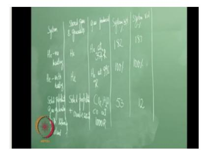
If you have helium with no heating right then the store gas is helium and helium at gas produced is also helium there is another scale of temperature called the ranking scale of temperature so this is in that unit then the weight is 180 2% then volume is 183 % now if we have heating right in the helium gas bottle itself helium is the stored gas and the gas produced is again helium at a higher temperature.
