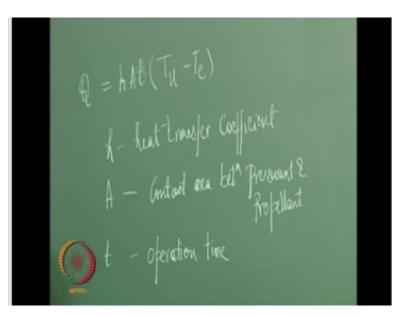
So you will get something like Q is equal to okay where h is the heat transfer coefficient right this is for a case wherein mostly there is a very little flow rate of the pressure and gas right is the contact area between pressure intent so plain okay then t is the operation time and te is repellent temperature and the U is pressure and temperature at the end of expansion now please remember that we are putting the pressure on tat a very high pressure in the gas bottle right.
