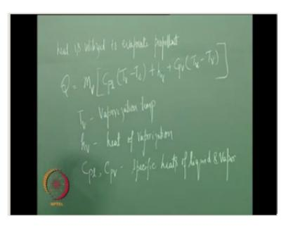
Now the same heat that is absorbed by the propellant causes it to evaporate right the propellant absorbs this heat and evaporates so, so if we have to calculate that so the same queue will be transferred to the propellant and it will lead to its evaporation remember the propellant is a liquid right so it has to change its temperature from its temperature to its boiling point temperature and then there is a constant heat of vaporization.
