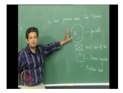
So after all this we know how, how much of mass of pressure and to be delivered and at what temperature and pressure right so fine now if you look at what is happening on the pressure and side pressure inside you have let us say a helium tank right and you have a valve here and then a regulator this is the and here it goes to the propellant tank right now if you look at what is happening inside this gas bottle.
