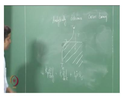
So analytically, so let us look at how to determine the burn rate analytically, now if you remember our burn rate equation for a solid propellant grain we are in this let us say this was the solid propellant and it is burning in this direction  $\dot{\mathbf{r}}$ . Now if you look at the temperature profile
