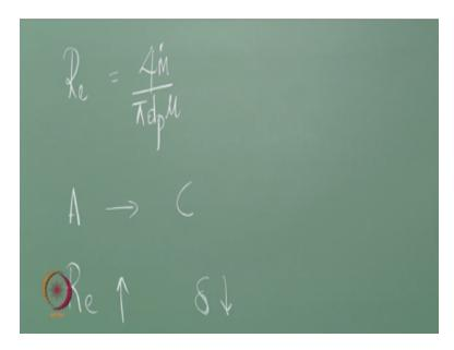
$4\dot{m}/\pi dp\mu$  where  $\dot{m}$  is the mass flow rate local mass flow rate, dp is the foot diameter and  $\mu$  is the coefficient of viscosity, so if you have this as you see mass when it gets added more the Reynolds number will increase. So as you move from A to C Reynolds number keeps on increasing and the  $\partial$  has a inverse relationship with Reynolds number that is as Reynolds number increases  $\partial$  will decrease.
