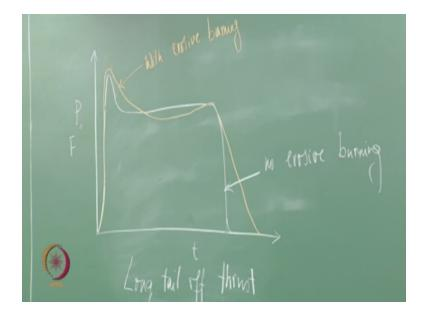
This could also be pressure comma thrust versus time, this is the line without a erosive burning and now if you super impose on the same graph the line with erosive burning, see if you look at the white line that is the line without any arrows you burning the pressure initially increases and drops to its equilibrium pressure and then remains there and the tail off is also very sharp, right.
