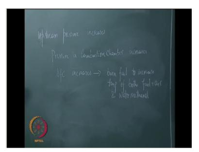
Now let us discuss the next method to increase the thrust of the turbojet that is water methanol injection now typically one would have added only water but methanol is also added because water at low temperatures that are encountered and the aircraft flies at high altitudes can freeze and that is an undesirable situation to be in.
