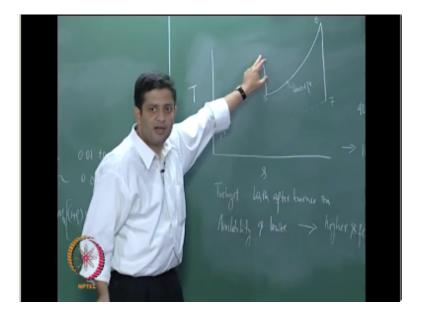
This is the TS diagram for turbojet with after burner on okay notice that earlier this was the maximum temperature that you were able to go up to because of the limitation so the turbine now if you are adding heat in the afterburner you can go to a much higher temperature but we need to remember one thing that we are adding heat at a lower pressure here this is lower than the main combustion chamber pressure.
