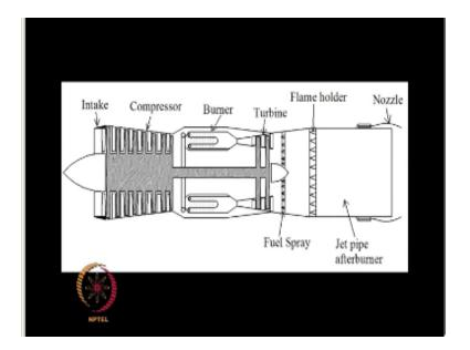
Now if you look at this turbojet engine here because there is a turbine you need to bring down the temperatures in the in front of it because turbine blades are only capable of withstanding a certain amount of temperature but there is also air that is in excess that is used here to bring down the temperature that is available for further fuel addition downstream.
