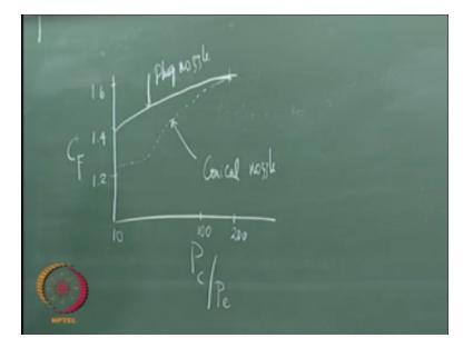
If we have  $P_C / P$  on the x-axis and  $C_F$  on the y-axis this is a log scale, so if you have a nozzle design for some high-altitude conditions and we are here a conventional nozzle or a conical nozzle will go like this whereas a plug nozzle will have a superior performance throughout this is okay, so the conical nozzle has a much inferior altitude at conditions other than the design conditions it is performance is not as good as a plug nozzle or a narrow spike nozzle, so next we
