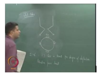
Now if we were looking at it from the bottom it would look like this now you could move this into the flow as per requirement okay and depending on the amount this up stretch the flow you will get the thrust force proportional to that okay, so as such this the both these do not obstruct the flow in their normal position, so they did not add to any loss in their normal operation but when they are used they will lead to a small loss with this you can get  $+ - 14^{\circ}$  of change in the thrust.
