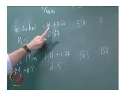
So this will again have two parts 1 point and at an altitude okay, this is what we see notice that as you go up in altitude the fraction of the pressure thrust is increasing it is a lower fraction here right or if you look at this number it is a lower fraction here compared to a higher fraction here right, the overall thrust why does this happen, why does pressure thrust part increase as you go up in altitude.
