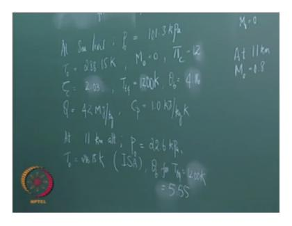
So firstly we will look at optimal, optimal expansion of flow in the nozzle here there are two conditions that we need to look at 1 is sea level thrust or sea level is been what happens at cruise conditions so at sea level P0=1 atmosphere 1011.3mPa and T0 to T if we assume an IS, IS a
