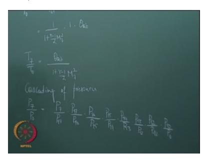
So I can get T7/T0 as Tt7.Tt6 by okay, Tt sorry this has to be Tt6 okay, fine these two cancel off and I will get T7/T0 what is T7/Tt7 it is the ratio of static to stagnation so I can express this in terms of Mach number this would be  $1+1/1 \gamma-1/2 m72$  what is T7/Tt7/Tt6 this is flow through the nozzle right.
