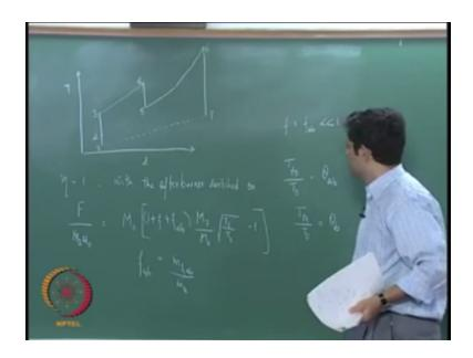
Now if we look at the TS diagram with the afterburner on we will again assume  $\eta$  to be 1 okay, so you have isentropic compression through the intake as well as through the compressor then you have heat addition in the main combustor expansion through the turbine so this is 0, 20kay, so this is the TS diagram for efficiencies 1 and with the afterburner switched on okay, now what do we have to do if you have to analyze this okay.
