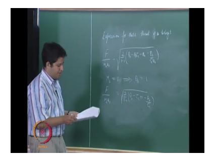
So you get okay so this is a nonzero quantity, so therefore we can safely say that whatever we have derived is correct and it produces nonzero static thrust okay, even when M<sub>0</sub> =0 what happens when M<sub>0</sub> = 0 what happens to  $\theta_0 \theta_0$  sorry when M<sub>0</sub> = 0 it means that  $\theta_0$  should be 1, so you substitute it here again you can rewrite this expression  $\theta_0$ . So this cannot go to zero and therefore we have a positive static thrust okay.
