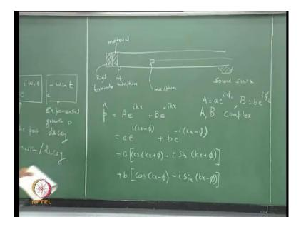
So, let me draw this picture once again, so we have, so this tube is the impendence tube and you have a sound source and you have a microphone. This is just symbolic of doing a throwers with the entire set up and as I mentioned you should have a reference microphone here. And you can either travels with a one microphone or you can put 20 microphones and get the acoustic field and you always need a reference to determine the phase.
