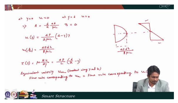
So, at y equal to 0, u is 0 and at y equal to d, u is 0 and that gives us the values of A and B and A becomes equal to d by 2 del P by mu L and B becomes equal to 0. So, after putting everything, mu of y becomes del P by 2 mu L multiplied by d minus y into y. Now if I want to find out the value of u at d by 2 by putting y equal to d by 2, the expression comes to be delta P d square by 8 mu L. Now if I plot it, the variation of the u with respect to y it looks like this.
