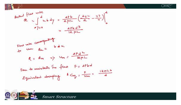
Now, Q the actual flow rate is equal to from y equal to 0 to d and that we can get by integrating this quantity and that gives us the flow rate as del P b by 2 mu L multiplied by d square by 2 minus y cube by 3 which is evaluated between at 0 and d are the limits.
