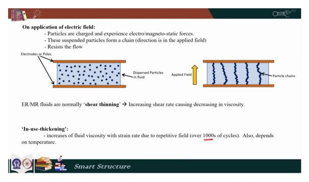
Again this shows the electro and magnetorheological effect. So, particles are charged. So, here it shows again the electro and magnetorheological effects this particle experience some force and because of the force, the alignment is done and its flocks the flow.
