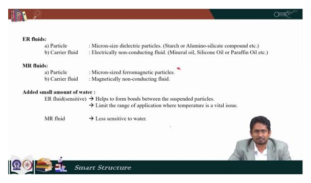
Now, here are some basic constituents. So, ER fluids have micron size dielectric particles like starch and amino silicate compound, electrically non conducting fluid like mineral oil, silicon oil, paraffin oil are the carrier.
