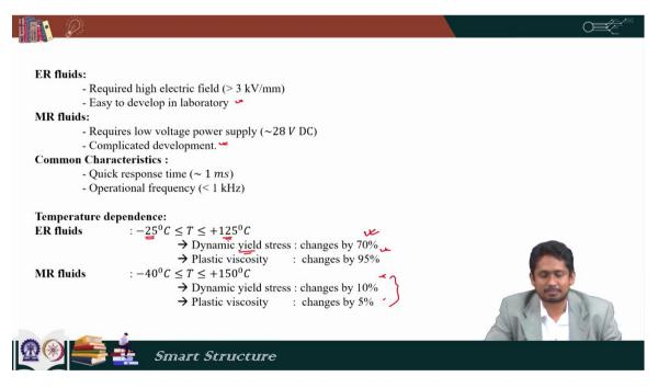
ER fluids generally require high electric field which is higher than 3 kilo volt per millimeter, but they are easy to form in the laboratory. MR fluids require low voltage power supply for example, DC voltage of 28 volt is ok for it that is why there is more focus on MR fluids now. However, their development is little bit more involved.
