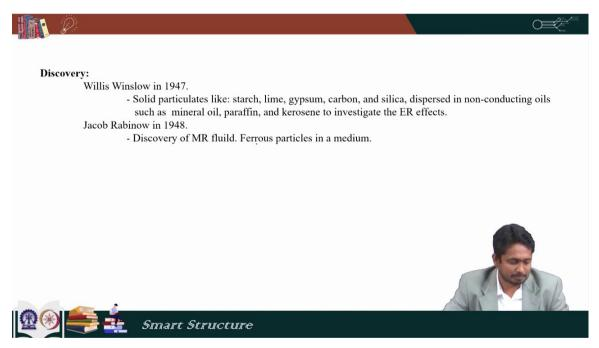
First in 1947 Willis Winslow discovered the electro rheological effect and that was discovered in a mixture of starch lime, gypsum, carbon and silica which were dispersed in non conducting oils like mineral oil, paraffin and kerosene. In 1948, the magnetorheological effect was discovered that was by Jacob Rabinow and that was seen in ferrous particles in a medium.
