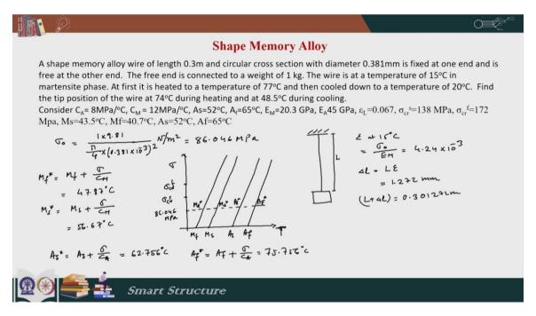
So, now we will first find out what is happening when we are at temperature 74 degree centigrade. So, to do that we have to find out the amount of martensite fraction and if I
