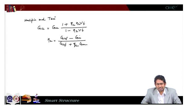
Now there is a equation by Halpin and Tsai for this case also and as per that equation it is Gm multiplied by in the denominator 1 plus Tsai two eta 2 Vf then divided by 1 minus eta 2 Vf where eta 2 is G 12f minus Gm divided by G 12f plus Tsai 2 Gm. So again we can experimentally find out Tsai 2 and we can fit the equation and we can use the same equation. Now this brings us to the end of this lecture.
