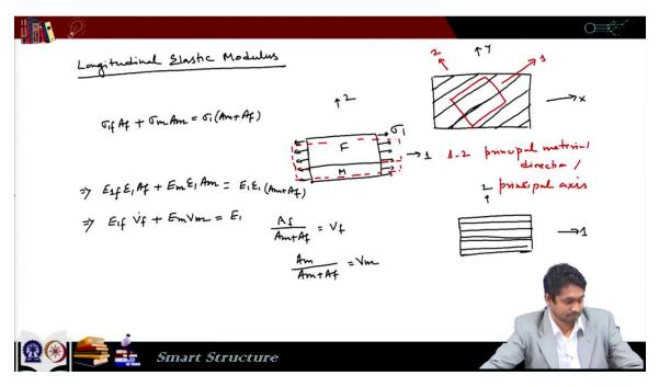
Now we will define the elastic properties. So let's talk about longitudinal elastic modulus. So our composite ply looks like this. We have plies oriented in some direction. Some theta its plies are oriented and our assumption is that they are aligned properly and spacing is uniform. So here we can talk about two axis one is let's define as x and y. So this is we can say it is a global axis and we can align one another axis.
