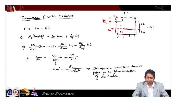
Now we will talk about the same properties in the transverse direction. In the transverse direction so we look at the same idealized diagram when it is loaded in the transverse direction. We have fiber here, we have matrix here. It is loaded in sigma 2 direction.
