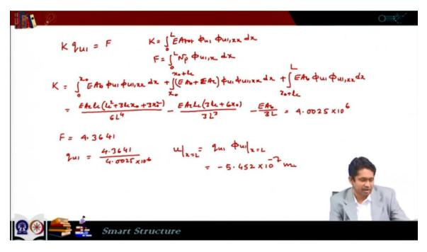
$$u(x) = \left(\frac{x}{L} - \frac{1}{2}\left(\frac{x}{L}\right)^2\right) q_{u1} + \left(\frac{x}{L}\right)^3 q_{u2}$$
