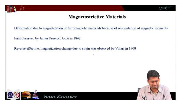
Now there is something called magnetostrictive materials and they are the magnetic counterpart. Here we get deformation due to magnetization of ferromagnetic materials because of reorientation of magnetic moments. It was first discovered by James Prescott Joule in 1842 and the reverse effect where magnetization change due to strain was also observed. That was by Villari in 1900.
