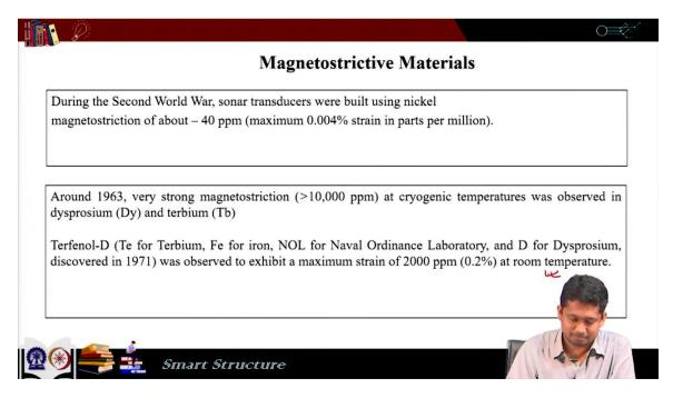
So, here we will see some applications of magnetostrictive materials. During Second World War, sonar transducers were built using nickel where we find magnetostriction of about 40 ppm. So, here maximum 0.004 percent strain in parts per million was observed. Then in around 1963, strong magnetostriction more than 10000 ppm at cryogenic temperatures was observed in materials dysprosium and terbium. So, there was a good amount of research in finding out materials which shows high magnetostriction.
