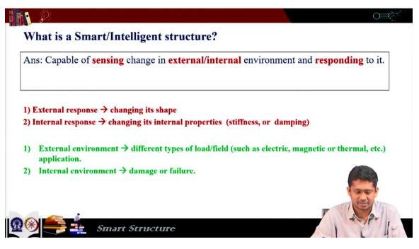
Smart structures are capable of sensing change in external or internal environment and responding to it. So, here we have two kind of conditions, one is external condition, one is internal condition. External condition refers to change in load or any external field like electric field, magnetic field, thermal field and so on.
