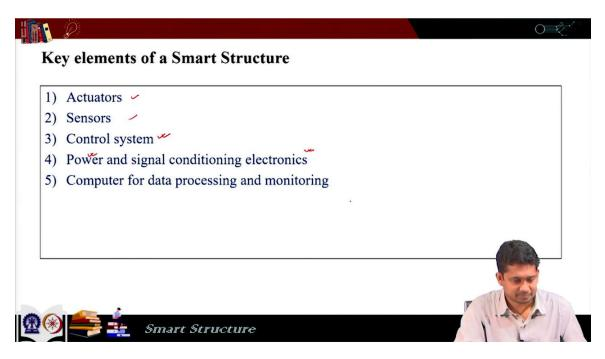
So, based on this discussion, we can say that we need quite a few components for smart structures. It needs actuators, sensors. It needs a control system. So, the control system takes the sensor data and then actuates power and signal condition electronics is needed. So, even in this power supply, some kind of smartness can be brought into. Nowadays with tremendous advancements in technologies, generally the sensors actuators and the associated equipments need much less power.
