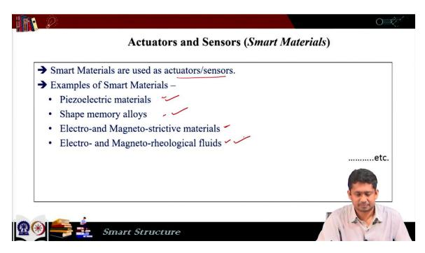
Smart material actuators and sensors as the name says, they are made of smart materials and smart materials have very unique properties which makes them good candidate for actuator sensor material. So, here are some examples of smart materials, piezoelectric materials, shape memory alloy, electro and magnetorheological fluids, electro and magnetostrictive materials and electro and magnetorheological fluids. So, in this course we will talk about these three materials in more details.
