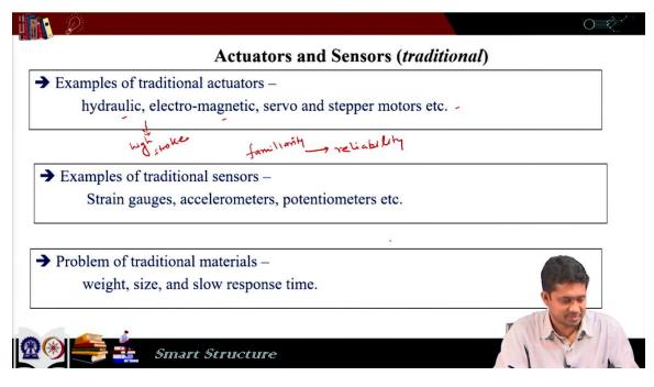
So, here we have examples of traditional actuators and sensors. Traditional actuators can be hydraulic actuators, electromagnetic actuators and servo and stepper motors.
