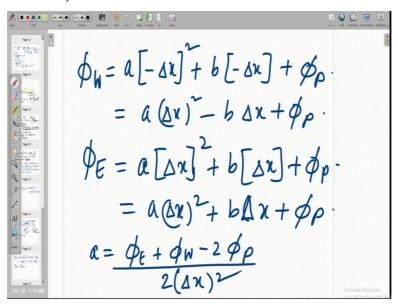
So, you will find that phi w is equal to a times - delta x square + b times - delta x + C which is phi p already. Now, this becomes a delta x square - b delta x + phi p. And then if we add the equations for. Okay. Before we add we write down the equation for phi E. So, for phi E, it will be this. So, we have, we do not have any negative signs here. So, that will help us to eliminate some of the unknowns and solve.
