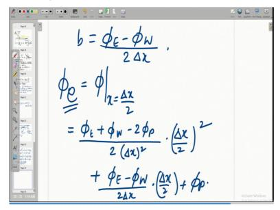
And then you can subtract the two equations and you can show b is equal to this. Right. And then what you need to do is substitute these a's and b's into the original equation and then rearrange the terms. After you do that what do you come up with, you come up with an expression like this. Okay.
