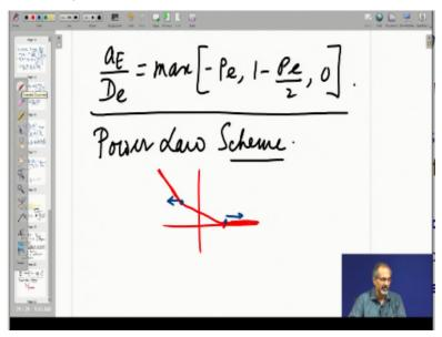
Now, this distribution can be written in a more convenient form, a more compact form which is very convenient for computer coding in this way. So, max of these arguments and you can check very easily that each one of these arguments when applied to the different 3 segments of the piecewise linear distribution, will give you the appropriate value for each portion. Alright.
