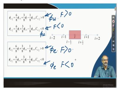
So, in this slide, you can easily see that for flow moving from left to right, this is how phi w can be worked out. From flow moving from left to right, this is how phi e can be worked out. So, this is F > 0, this is F > 0, and these are for F < 0. So, this is the phi w expression for F < 0. Again, phi e expression for F < 0. So, from that one equation that we have worked out now. We can actually derive all these equations just by shifting it by half cell width. Right.
