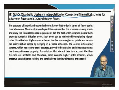
But at the expense of more computing effort. That scheme is called as the QUICK scheme, Quadratic Upstream Interpolation for Convective Kinematics, which uses quadratic fit involving 3 nodal points to calculate the values of phi at a particular cell face. So, let us do calculation on how QUICK scheme works. Before we do that will just put a small grid together.
