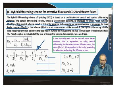
So, hybrid scheme as we said earlier that it is a combination of central and upwind differencing schemes and it is one in which diffusion is set to 0 when Peclet when cell Peclet number exceeds 2 and you can actually calculate the fluxes at the faces using distributions of this form. In the derivations, we have talked about how the coefficient a E by D e functions for a hybrid scheme.
