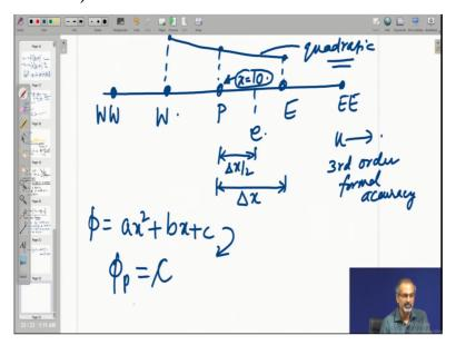
And show the different points which are of importance to us. So, let us say, we want to compute the value of phi at the point e and the velocity is moving from left to right. In the case of QUICK, what we do is, we take 3 nodes and make a quadratic fit; making sure that we have taken two upstream nodes and one downstream node in the process.
