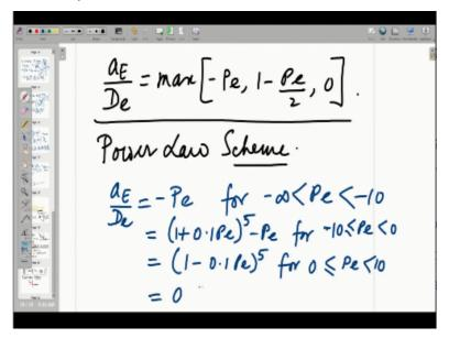
Now, if you do that what does it come to? What does the scheme come to? Let us try to define the scheme straightaway. So, for the Power Law scheme, the cutoff Peclet number happens to be 10. That means, on each side + or - 10 and the intermediate portion is patched not by a straight line, but rather a Power Law distribution which you can clearly see from this functional form which I am currently writing.
