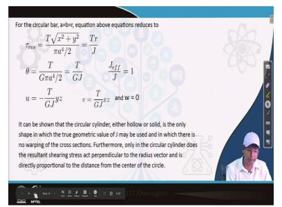
For the circular bar where a is equals to b is equals to r so we come back to the simplified solution considering a and b are equals and is equals to r and we will try to see observe that the derivation whatever we have done that also holds for a circular section that is what is done a is equals to b is equals to r is put here and the tau resultant shear stress if we put those values is equals to t r by J and the theta is T by G J and J effective is also equals to J and it is equals to 1.
