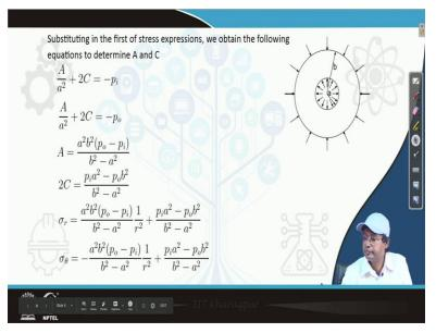
Substituting the first of stress expression we obtain the following equation to determine A and C. So in sigma r if we substitute we have this is equals to p i and this is also a this is say mistake
