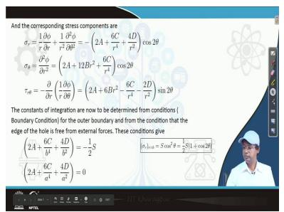
So what we need to do is that and the corresponding stress components sigma r since we have got that stress functions with constants A B C D if we use the stress function expressions with to find out the normal sigma r and sigma theta and tau r theta we get these components as minus of 2A + 6C by r 4 to the power 4 4D by r square cos 2 theta sigma theta is in this function these are the fr portions and then we have this form also.
