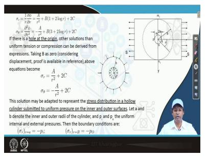
So what we have consider here is that we are there is a hole of diameter twice a uniform tension is acting of amplitude S we are considering one more circle b which is considerably large in red in radius in comparison to the whole radius. And we are assuming that the stress distribution beyond this hole beyond this circle is a uniform, uniform in the sense as if there is no hole in the structure or the plate.
