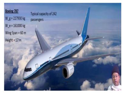
Another dream machine they say is Dreamliner 787 Boeing. So the wingspan is noticeable as 60 meter height is about 17 meter and typical capacity is about 242 passengers. So this is again having engine is reduced here. Again number of engine reduces because of the advance in the or progress in the engine technology, size of the engine, more latest engines are used and that way it gets reduced.
