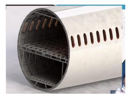
This is another view, another SolidWorks drawing or CAD drawing I must say, previous also is a CAD drawing. This view is different. In this view, these bulkheads are quite clear. This is the beam. We always put holes in the beams to reduce weight. In this structure also you see there are holes to reduce weight and we will see why this window shape has come, what was the reason why stress is important around this hole.
