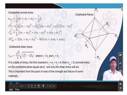
So the octahedral stresses we have this is what we have and the tau the shear stresses the normal stress is this and the shear stress we can find out substituting the values of direction cosines in this equation. And what we can find out that the tau is equals to this and in do simple maths we have 9 tau octahedral shear stress square is equals to 2 into i square or the first invariant square plus 6 into this is the second invariant.
