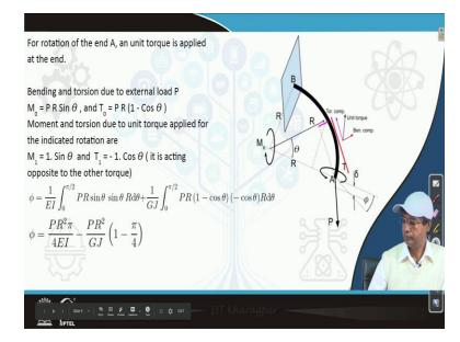
So here we have considered some additional drawing we have prepared for better understanding. What we need to see is we need to apply one torsional load, torsional unit load in the direction of in the direction where the theta is increasing and accordingly we can find out whether it is what is the value of Phi or the end rotation. So, for the rotation of end A and unit torque is applied at the end bending and torsion due to external load T.
