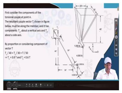
First about the torsion components first consider the components of the torsional couple at Point A here. The resultant couple vector T shown in figure below must be along the member. So, it is along the member as I showed you in the last slide and it is it has components  $T_V$  about vertical axis and  $T_S$  about the side axis. This is please you may note that this is vertical axis this is dragged access this is side axis.
