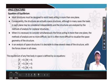
As a general introduction let us try to get introduced with the problem equation space structures. Equations of equilibrium is most necessary thing we need to find out the equation equations of equilibrium to solve problems. Most structures must be designed to resist loads acting in more than one plane this is what I was telling you a few minutes back. But in general we reduce it to a plane structure so that problems becomes easy.
