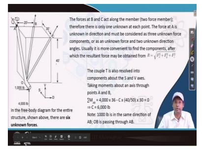
So, here we have a relation between components of torsion those components are shown in this figure. Here all the unknowns are also shown as I mentioned there are three forces acting on a and we need to find out those forces and let us see slowly how do we get as I mentioned previously that in the free body diagram for the inter structures shown over there are six unknown forces. So, six unknown forces are these are components do not take it that way the torsion is the unknown.
