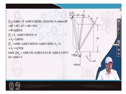
So we are considering equilibrium in the drag direction solution of  $F_D$  equals to 0. If we consider summation of  $F_D$  equals to 0 ( $\sum F_D = 0$ ) it gives us the force B because in this direction this is known these are orthogonal to that direction whereas this will have a component in that direction this also will have a component in that direction but we we have already found out this force this is known force that is 6000.
