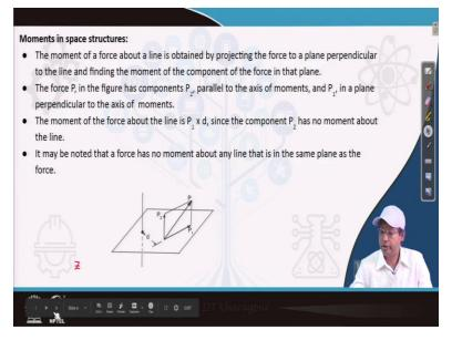
How to take moment consider moment that's a really important issue we need to learn moment in space structure. The moment of a force about a line is obtained by projecting the force to a plane perpendicular to the line and finding the moment of the component of the force in that plane. Apparently there are two things I should mention about a line. In two dimensional plane frames structures we were taking moment about a point not about a line.
