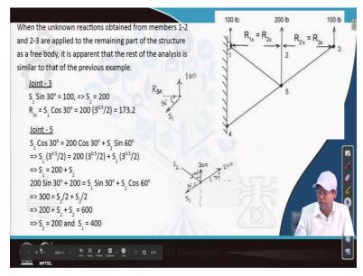
When the unknown reactions obtained from member 1 2 and 2 3 are applied to the remaining part of the structure as a free body. It is apparent that the rest of the analysis is similar to that of previous example. So, it is almost similar to the previous example as it is said those forces are applied here as shown here and then considering joints one after another we can easily find out the forces. So, first this joint is considered so  $S_1$  we are keeping the name here as  $S_1$ .
