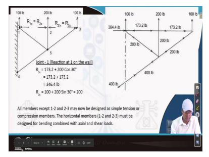
This slide is about joint one reactions at one on wall we need to find out here this 400 pound is already known because this is pin joint and it is a two Force member this is already known one the reaction here we need to find out reaction at one that is the reason it is stated reaction at one on the wall. So, R OX or 0X sometimes we say, reaction is we are considering this as 1732 is that this member force already you have found out, those are equal.
