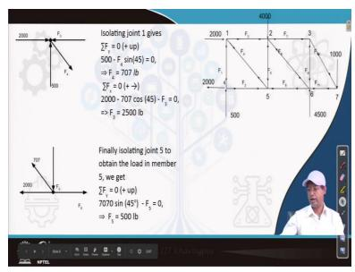
So, once we have found out the joint 4 see this member force is already known. So, if we consider this joint here the unknown forces are this and this. So, we have two equations easily we can find out these two member forces that is what is done here in this the joint  $F_3$  is taken as a kept aside free body diagram of that joint 3 is prepared 500 is the  $F_1$  force is applied here external force 2000 pound is applied there.
