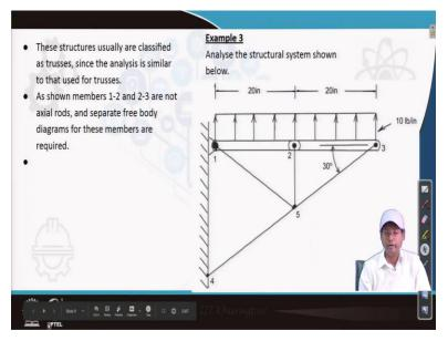
So we will have solved two problems, two problems one in one method the other one in two methods and this one is not exactly our principally truss but we can solve this problem considering truss concept and let us see how do we do. Because in general the truss members are not loaded transverse to its axis. So, but in this particular case this member and this member is loaded transverse to the this axis in the upward direction.
