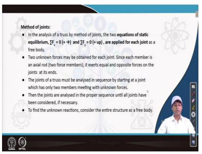
Method of joints if we look at in this analysis of our truss by method of joints the two equations of static equilibrium that is horizontal forces are  $\sum F_x = 0 \ (+ \rightarrow)$  and vertical forces  $\sum F_y = 0 \ (+ \mu)$  are applied for each joint that is the reason each joint gives us two equilibrium equations. We need to consider the free body and then we need two free body of that particular joint and it reapply these two.
