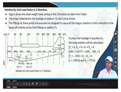
Solution for unit load factor in Z direction, figure shows the deadweight loads acting in the Z direction as taken from table. This values it is talking about all these values 893 pound at station 11, 388 pound at station 50, 307 pound at station 80, 120 at station 120, 407 at station 170, 311 at station 200, 176 pound at 230 station 230 it is 10 pound 260, 21 pound at station 290 it is 118 pound at station 315 it is 22 pound.
