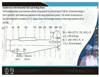
This is for the unit tail plane solution for unit horizontal tail load acting downward 275.5 is the station value that is there is in 100 277 -73 this about this point when the moment is considered as the reason this is the station point value how far it is from this section and load is 100 the fuselage shears and moments will be computed for a unit even a tail load of 100 pound.
