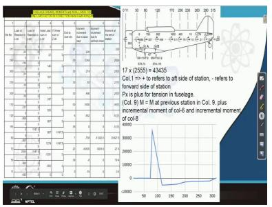
And this table also is there is not much things to explain because already we have explained one table. Only difference is that here we have one more moment component that we need to see moment increase due to axial load, moment increment due to vertical shear, moment at the left of
