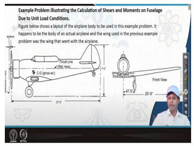
So our example is this aircraft this is a text book problem we have already solved the wing for bending moment and shear force. Example problem illustrates the calculation of shear and moments on fuselage due to unit load condition. Will cover the shear and moment in future class but that starts here that is why it is stated here. We will only do in this lecture that distribution and re distribution of the loads coming on the fuselage and how do we need to carry out that for unit load analysis.
