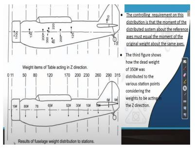
Let see the controlling requirement on this distribution is that the moment this already we have read so I am not going to read again thus for reference to this slide it is put down there. The third figure shows how the dead weight of this how the dead weight is distributed. All this mainly the 350 load this load is distributed at station 11 as 19 pound 80 pound 78, 65 all this way this has been done.
