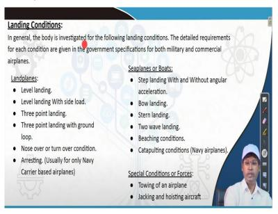
Landing condition as I told you landing condition is very critical condition. In landing condition in general the body is investigated airplane body is investigated for the following landing conditions. The detailed requirements for each condition are given in the government specification for both military and commercial airplanes. So certifying agencies generally give this different; certifying agencies for different condition for land planes.
