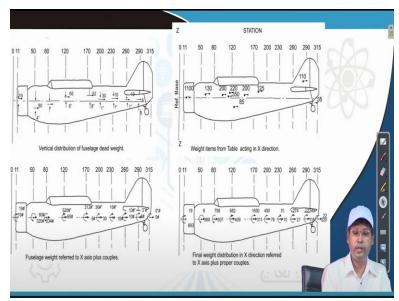
Ok this is we have concepts in how it is distributed in in the vertical direction. This figure shows in the horizontal way how it is distributed 80 is acting here. This is the mistake the corresponding values is not put there you may please refer to the table. 65 is acting above the X line 52 is acting above the X line, and similar way on the X direction where the loads are acting all those things are shown here.
